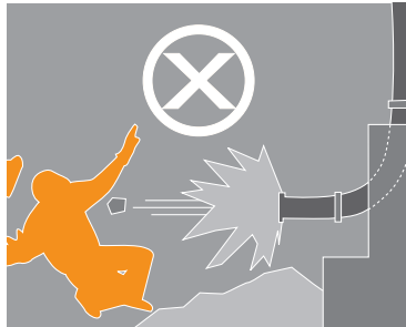
Keep clear of discharge end of pipe
