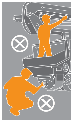
Dangerous cleaning practices
