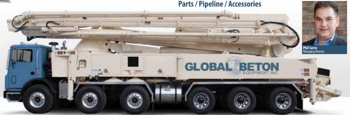
We can provide placement booms for your truck mounts or provide ready mounted booms on Mack or TOR chassis.
